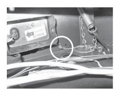
Connect one end of the supplied green ground wire to the lug with the nut and washer from the kit.
